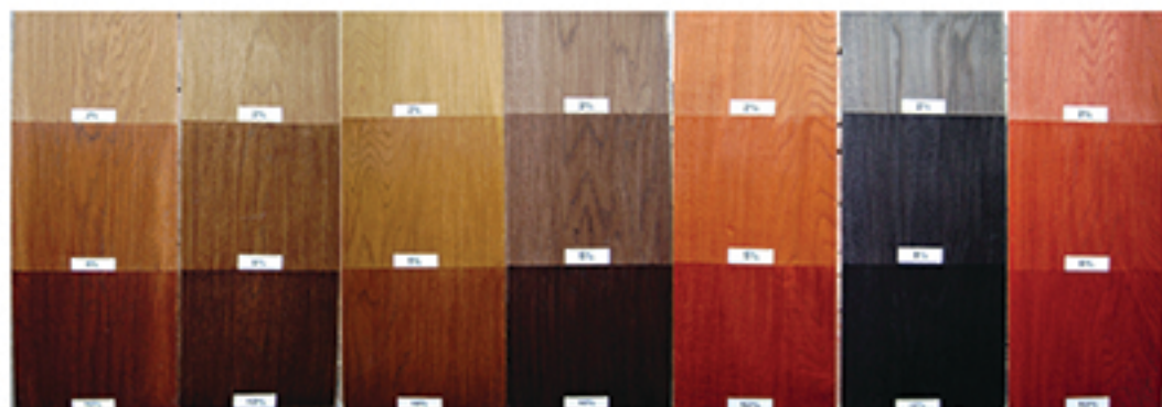
Some examples of Tingo Universale added into Fondo Impregnante B/C in different ratios.
